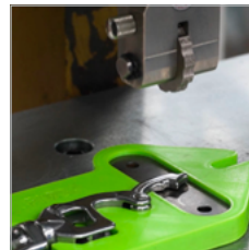
Stamped with production code for traceability
